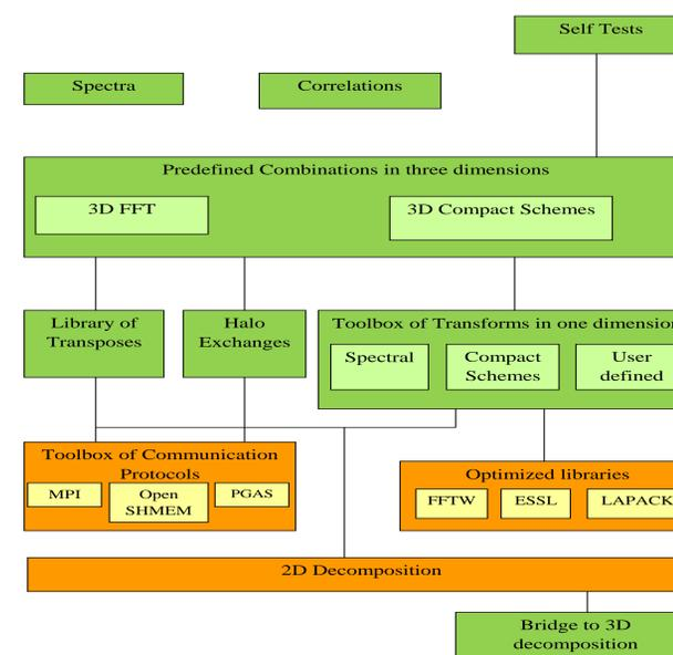
**Figure 3.** Structure of proposed software package. It will be built on top of well-optimized libraries such as FFTW, ESSL, LAPACK, and will be based on 2D domain decomposition. It will be built in a modular fashion providing flexibility to the user.
