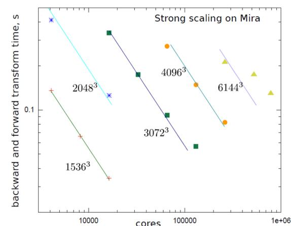
**Figure 1.** Scaling of P3DFFT on IBM BG/Q "Mira" at Argonne National Lab (A. Beresnyak).
